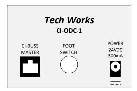
The CI-ODC-1 is an Operator Desk Console Intercom that includes a professional 12 inch cardioid gooseneck microphone and a moisture resistant 45 ohm speaker. On the side of the console is an industry standard RJ-22, telephone handset connector to accommodate a Plantronics Wireless Headset (Sold separately).
