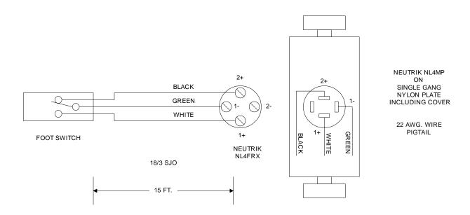
Typical connection for a call switch is to use the normally open contact or Green and White wires. This would also provide a Push To Talk function.
