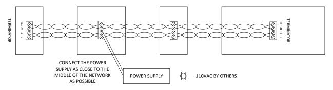
Due to the implementation of innovative data noise canceling circuits in all Tech Works RS485 microprocessor products, the data and power can now be run in any direction up to a total wire length of 3000 feet.
