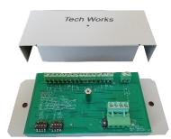
The Tech Works **CC2-CM-Z** is a Zone Output Control Module designed to work with Tech Works Intelligent Networks. Units are equipped with screw terminals capable of supporting up to four light outputs. The **CC2-CM-Z** is a surface-mounting device constructed of cold rolled steel with a removable cover plate and is designed to provide LED outputs for Zone Lights and an Alarm contact closures output.
