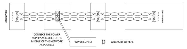
Due to the implementation of innovative data noise canceling circuits in all Tech Works RS485 microprocessor products, the data and power can now be run in any direction up to a total wire length of 3000 feet.
