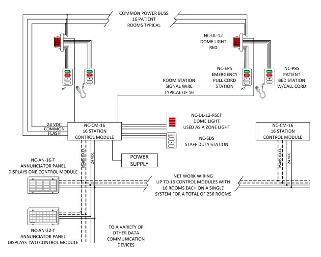
The Dome Light uses discrete logic to control the patient room stations and indicate their status through LEDs. The Dome light then uses the single conductor annunciator wire to communicate with a Digital Control Module. The Control Module then converts the simple logic from the Dome Lights to RS485 communication to share the status of all room dome lights with other RS485 smart annunciators and bridges to other communication protocols.
